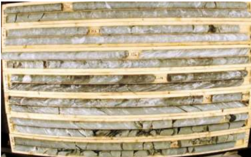
Figure 10-6: CD-3 from 119 m to 140 m. Typical core from the condemnation holes around Lac Denis
