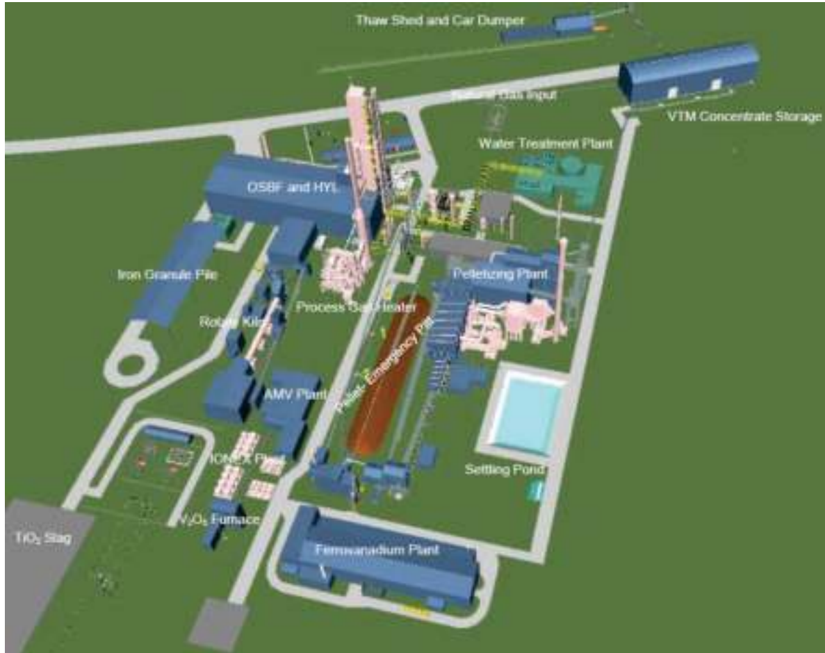
Figure 18-17: Overall layout of the BRM Metallurgical Plant
