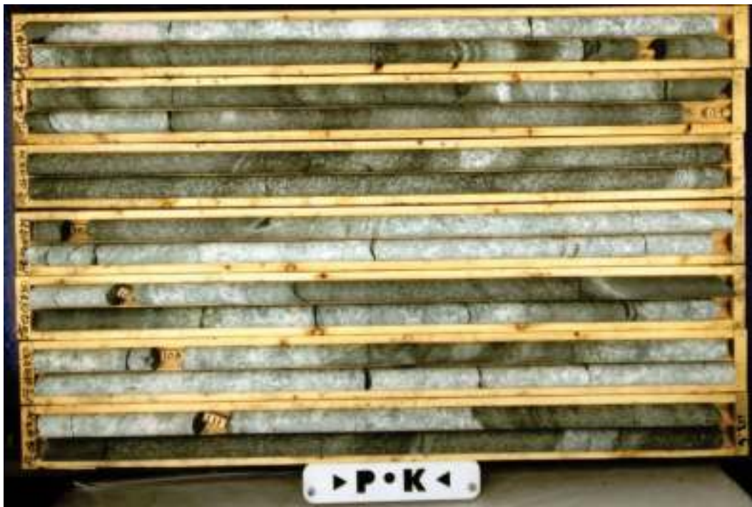
Figure 10-4: Example of PK scanned core AE-02-01, 94.5 m – 113.3 m. This is Part of the Virtual Core Shack that Encompasses Core for Essentially the Entire Project
