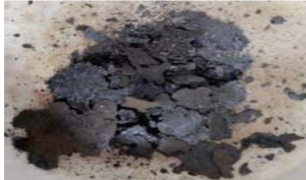
Figure 13-22: Contamination from the metal crucible
