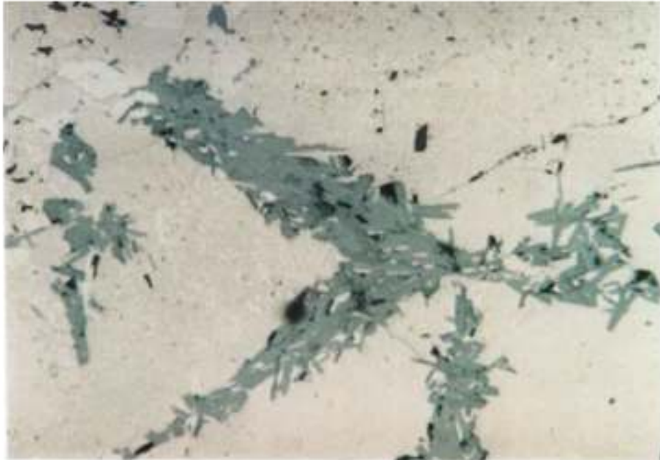
Figure 9-12: Decussate Structure of Chlorite (dirty green) along Alteration Fractures in Magnetite (pale grey).
